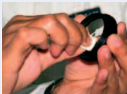
Figure 3. Always handle loose optical components by their edges. Clean round optical surfaces from the centre to the edge in a widening spiral.
